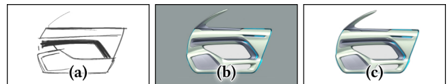
Figure 8: Generating components. When the designer presses a keyboard shortcut, the system (a) captures each component sketch in the orthographic view, (b) generates renderings from the sketch, and (c) applies background removal [14].
