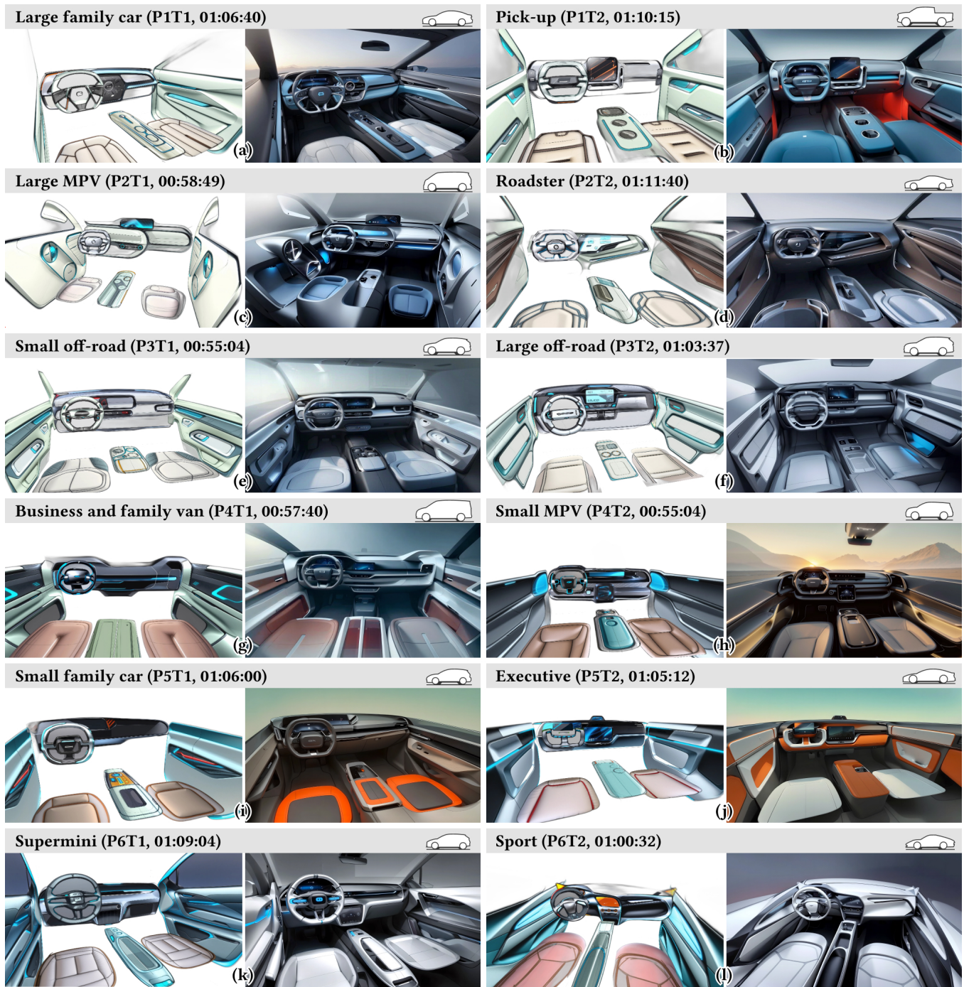
Figure 11: The final pre-visualizations (left) and renderings (right) produced by the designers in the user study. (a) A large family car by P1. (b) A pick-up by P1. (c) A large MPV by P2. (d) A roadster by P2. (e) A small off-road by P3. (f) A large off-road by P3. (g) A business and family van by P4. (h) A small MPV by P4. (i) A small family car by P5. (j) An executive by P5. (k) A supermini by P6. (l) A sport by P6.
