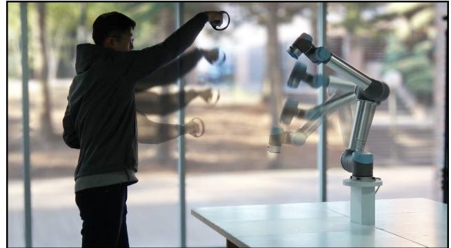
Figure 1: Robot Telekinesis [Lee et al. 2020] allows the user to remotely control the movement of the end effector of a robot arm with hand gestures that closely resemble handling a physical object.
