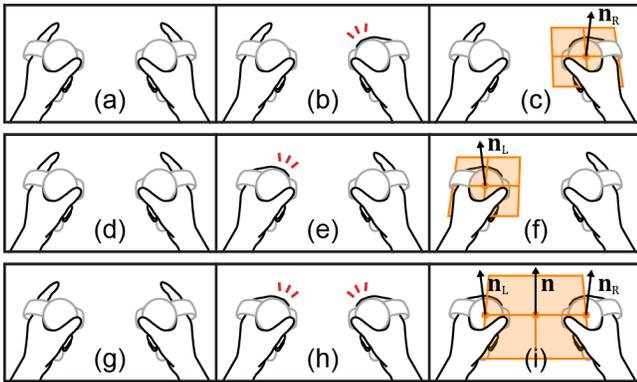
Figure 2: (a, d, g) The user holds two 6-DOF controllers. When the user activates (b) the right or (e) the left controller, a virtual plane with the normal (c)  $n_R$  or (f)  $n_L$  fixed to the controller is created. (h) When the user activates both controllers, (i) a virtual plane is created whose center is the midpoint between the two controllers, primary axis is the line segment between the two controllers, and normal  $n$  is the average of  $n_R$  and  $n_L$ .
