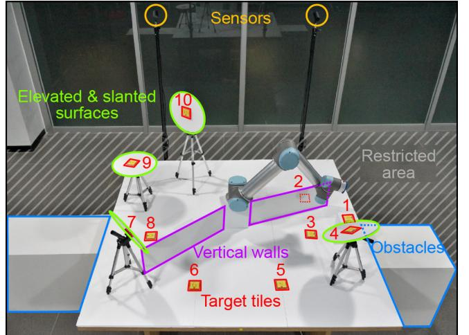
Fig. 6. Workspace setup. Using the above techniques, participants picked up 10 numbered magnetic tiles (red) in ascending order. Various fixtures (purple, green, blue) introduced additional elements of challenge.
