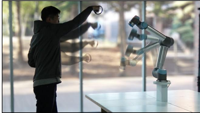
Fig. 1. Robot Telekinesis lets the user remotely control the movement of the end effector of a robot arm with hand gestures that closely resemble handling a physical object.
