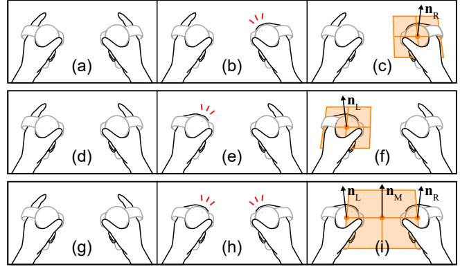
Fig. 2. (a, d, g) The user holds two 6-DOF controllers. When the user activates (b) the right or (e) left controller, a virtual plane with the normal (c)  $\mathbf{n}_R$  or (f)  $\mathbf{n}_L$  fixed to the controller is created. (h) When the user activates both controllers, (i) a virtual plane with the normal  $\mathbf{n}_M$ , the average of  $\mathbf{n}_R$  and  $\mathbf{n}_L$ , is created at the midpoint between the two controllers.
