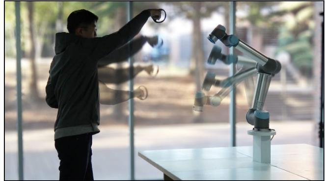
Fig. 1. Robot Telekinesis lets the user remotely control the movement of the end effector of a robot arm with hand gestures that closely resemble handling a physical object.
