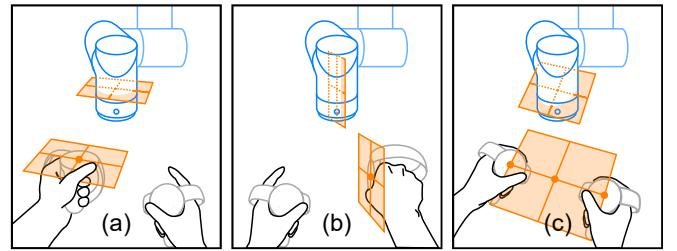
Fig. 3. When a virtual plane is created at (a) the left hand, (b) the right hand, or (c) the midpoint between the two hands, another virtual plane with the same orientation is created at the center of the end effector of the robot arm. The handheld plane acts as a motion proxy to the one at the end effector.
