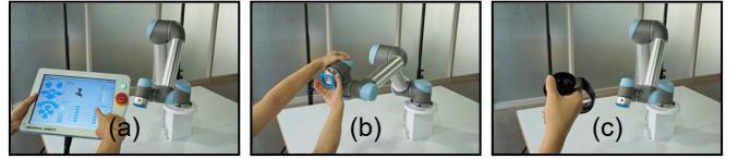
Fig. 5. Formal evaluation compared two baseline techniques: (a) teaching pendant (TP) and (b) direct teaching (DT), against (c) Robot Telekinesis (RT).
