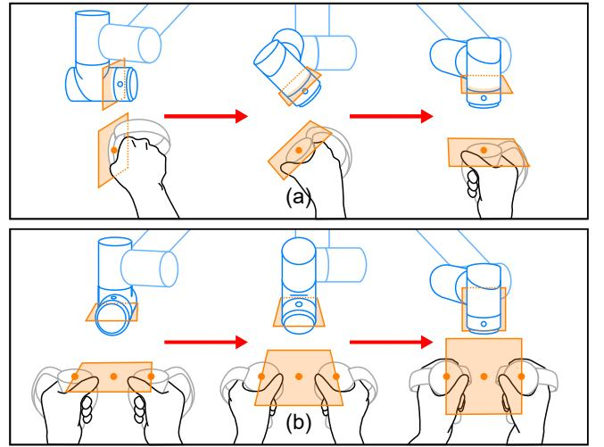
Fig. 4. When the handheld virtual plane is translated and rotated, the motion deltas of the handheld plane are transmitted to the end effector in real time. The user can thus control the end effector, as if physically holding and moving it by the planar handle, with (a) one or (b) two hands.
