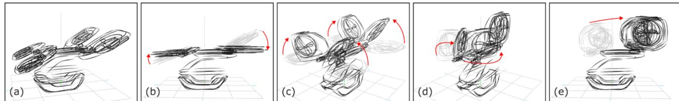
Figure 13: (a) A 3D sketch of a concept flying-car produced with our system. (b-e) The four thrusters perform a series of maneuvers to become fully folded after landing.
