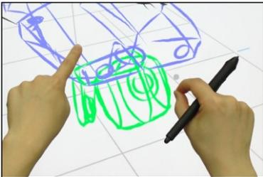
Figure 10: In our system, for inverse-kinematics posing, the designer uses one finger touch-and-hold (left hand) and a mid-air pinch gesture (right hand).
