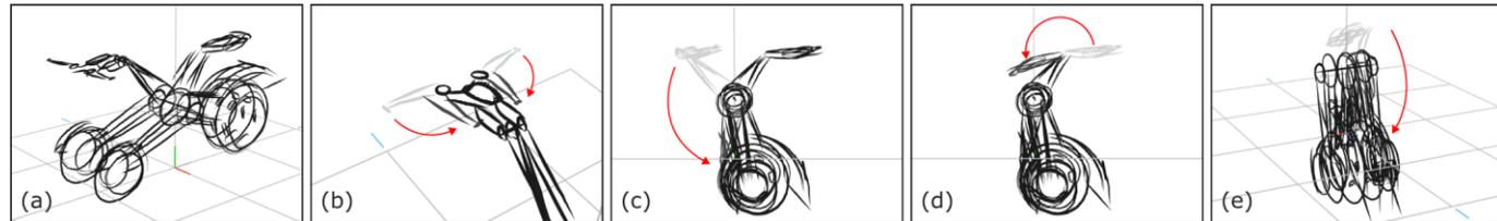
Figure 12: (a) A 3D sketch of a concept foldable e-bike produced using our system. Sequentially, (b) the bike handle, (c) the front of the bike, and (d) the back of the bike are folded into (e) the portable form.
