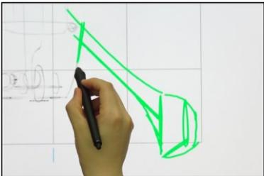
Figure 7: In our system, the designer makes a layer tab, marks curves, and trims them using precise and rough erasers, into separate parts.
