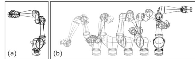
Figure 2: Using our 3D sketching system for multi-pose products enables (a) a static 3D sketch with chained moving parts to be (b) easily posed, allowing designers to focus on ideating, iterating, and communicating multi-pose product concepts.
