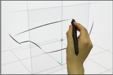
Figure 6: In our system, the designer sets up reference geometries, such as a 3D plane, and then sketches on them.
