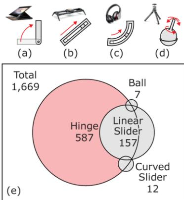
Figure 4: Across all 637 multi-pose products, only 4 types of joints were observed: (a) hinge joints, (b) linear slider joints, (c) curved slider joints, and (d) ball joints. (e) A Venn diagram, showing the number of times these joints appeared in the surveyed products. Shaded area (pink) shows that a large portion of products rely entirely on hinge joints.
