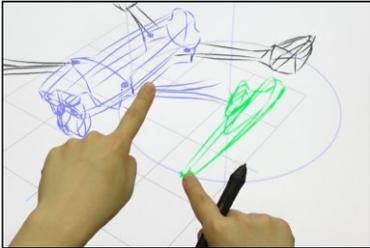
Figure 9: In our system, for forward-kinematics posing, the designer uses one finger touch-and-hold (left hand), and one finger touch-and-drag (right hand).
