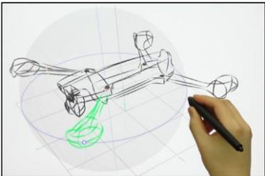
Figure 8: In our system, the designer draws a circular trajectory on a 3D sphere to indicate a rotational motion by a hinge joint.
