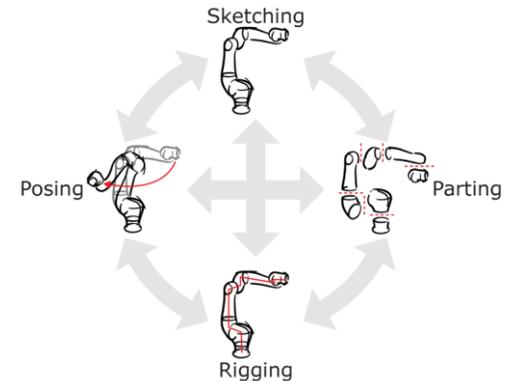
Figure 5: Using our system, the designer performs sketching, parting, rigging, and posing, to ideate and iterate on multi-pose products. These activities can be performed in any order and repeated any number of times.
