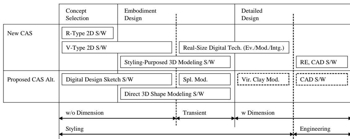
Figure 2. New CAS flow and proposed alternatives
